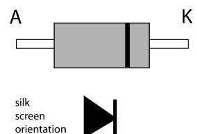
The diode must be oriented correctly. There are two ends, anode and cathode. Be sure that orientation matches the silk screen.
