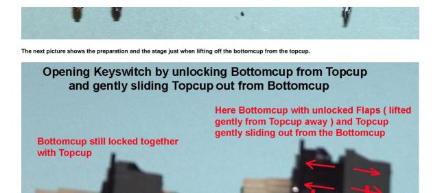
The next picture shows the parts after they have been extracted from eachother and the view of the parts visible then....
