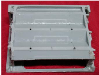
**11)** Get the battery box cover plate from an NXT. Remove some of the interior structure to accomodate some nuts and washers for attachment to the modified PowerFunctions battery box. Screw the partially completed PF box to the NXT lid using 2-56 screw hardware, 4 hex nuts, 4 washers and 4 flat-headed, phillips screws 1/4"(?) long. For now, unscrew and seperate the two components.
