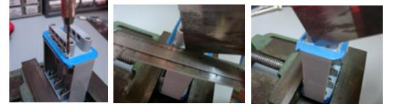
4) Unscrew and remove interior battery box, by sliding away from switch assembly/chasis.
