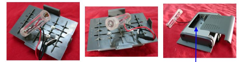
Load the "spare", self contained faux battery into the most recessed battery recepticle in the new battery box. Your new NXT battery box expansion is now ready for use with 1.2 volt rechargable batteries~
